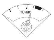
For vehicles with a turbo gauge, it indicates when the vehicle is using turbo power.
